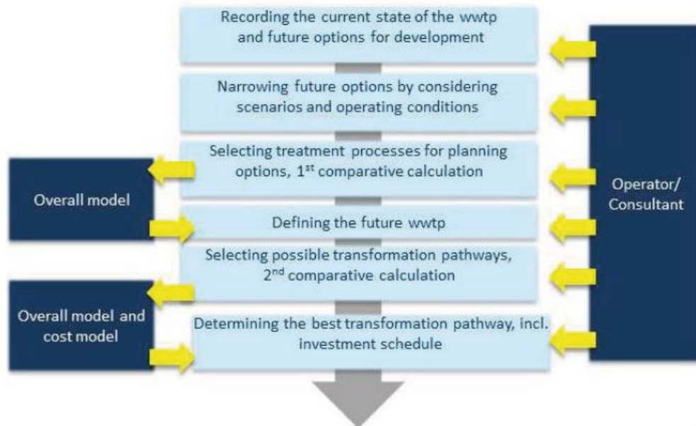
Fig. 3: Operating procedure describing the interactions between model use, results evaluation and the transformation process
